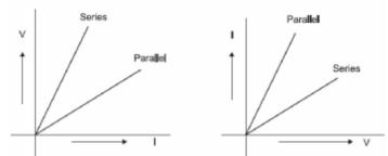
**Ans.** Both are correct because  $\Delta V/\Delta I$ = resistance(R) and AI/AV=1/R Series means high resistance and parallel means low resistance.
