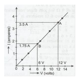
Resistance of resistor (R) =  $V_A$ - $V_B$ / $1_A$ - $1_B$  = 12 V - 6 V/ 3.6 A - 1.8 A
