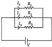
The current flowing through the two resistances in parallel is, however, not the same. When we have two or more resistances joined in parallel to one another, then the same current gets additional paths to flow and the overall resistance decreases.
